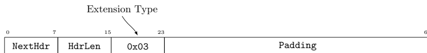
Figure 15.9: The header of the one-hop path extension. It is a hop-by-hop extension, thus the preceding NextHdr field has value 0x00.
