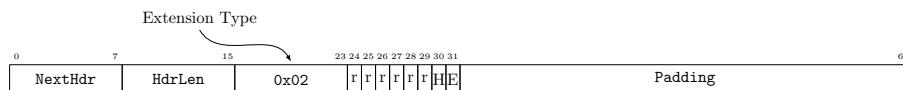
Figure 15.21: The header of the SCMP extension. It is a hop-by-hop extension, thus the preceding NextHdr field has value 0x00 .
